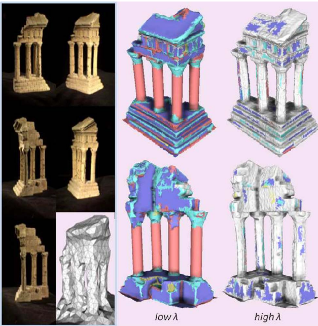
Fig. 12. Impact of the \lambda coefficient from the Temple dataset. Left: Input images and a rough visual hull as initial surface; center: result with a low \lambda value; right: result with a high value. Color code: See Fig. 7. The lower the value of the \lambda parameter, the higher the primitives to mesh-patches ratio in the final result. The high \lambda version has 0.48 mm accuracy and 99.7 percent completeness on the Middlebury benchmark [18], whereas the low \lambda version has 1.03 mm accuracy and 95.7 percent completeness. Note that the reconstruction of columns and pieces of walls by cylinders and planes engenders a loss of accuracy in such a case, i.e., when the structures are not regular.
